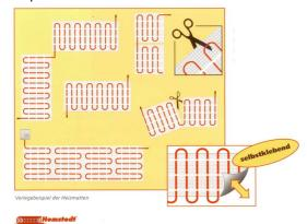
Important! Do not damage the heating cable. Bend the heating map where you cut it and install it in parallel with the first web.
