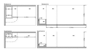
Figure: Areas without heating mat around bath tubs and shower trays
